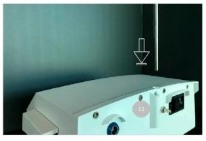
G. Align and attach the bracket to the housing provided on the console's rear (11) and suspend the irrigation solution flask or bottle FIG. 4.
